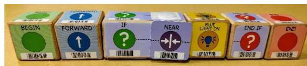
Figure 3. This figure provides an example of a conditional statement with KIBO.
