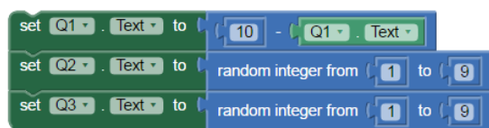
Figure 10. A logical error in the design of codes in always getting a sum of 10 from two of the three random numbers.
